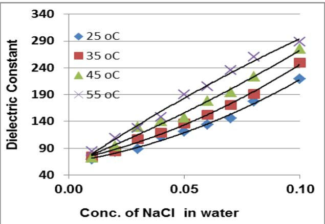
Fig. 4 Variation of dielectric constant of NaCl in water
