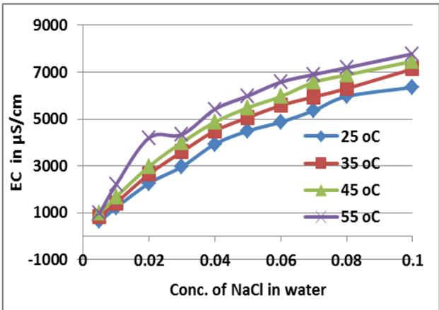
Fig. 3 Variation of Electrical Conductivity of NaCl in Water
